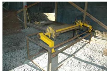
*Mesh bender: The NGA designed and built mesh bender*
