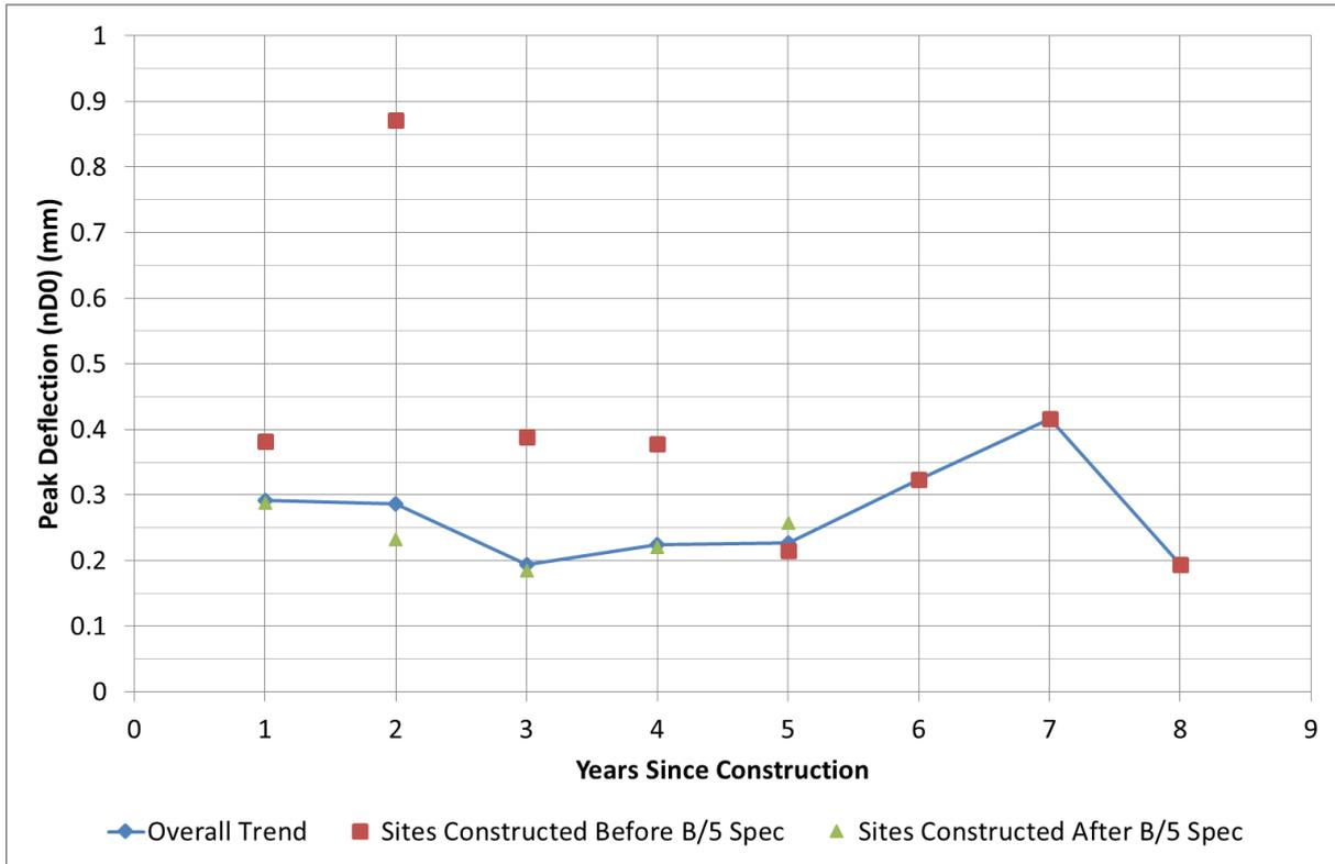
FIGURE 2: MEAN NORMALISED MAXIMUM DEFLECTION BY YEARS SINCE CONSTRUCTION
