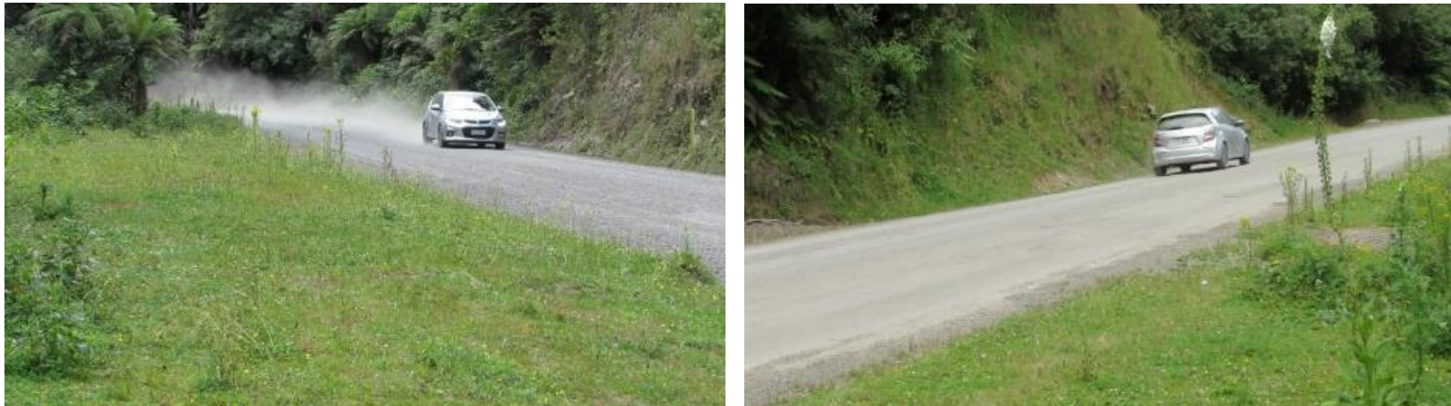
Left: visible dust behind the vehicle on untreated section, Right: minimal dust behind car on the trial section
